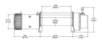
Rated Line Pull: 4310 kg single-line Motor: 12V 4.48kw, High output parallel series wound Remote Control: Remote switch, 3.7m lead Rope: Steel -- 30m, 8mm diameter Weight: 39.5 kgs
