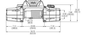
Rated line pull: 5443 kg single-line Motor: 12V DC, series wound Remote Control: Remote switch, 3.7m lead Weight (kit shipping): 44 kg Rope: 9.52mm x 24.38m steel
