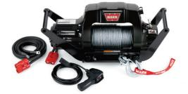
Rated line pull: 4310 kgs. single-line Electrical controls: Contactor Remote Control: Remote switch, LED indicator, 3.7m lead Drum diameter/Length: 6.4cm/23cm Wire rope: 38m, 8mm diameter
